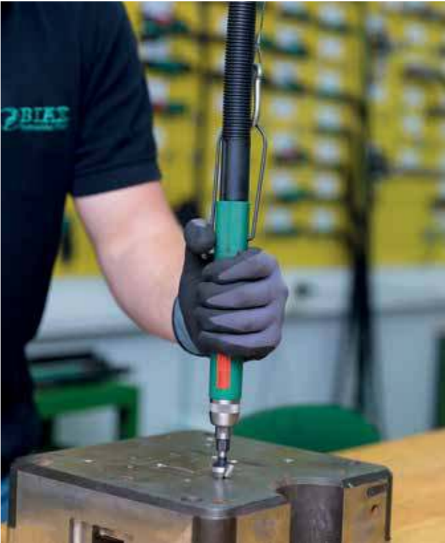
All straight drilling deburrers can be operated with a spring balancer.
