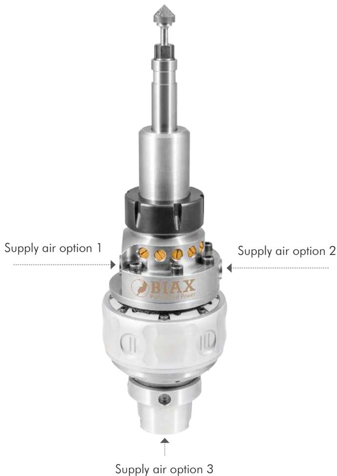
Whether you use a HSK or SK mount, we have the most common types of mounting in our programme. If you need a mounting that we do not currently offer please contact us. The RSC system can be driven with compressed air through the internal coolant system of the CNC machine. There is no requirement for manually installing any hoses or cables.
