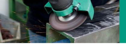
The WRD/H 10-20/3 S from BIAX is the smallest and lightest angle grinder for grinding discs on the market. The device can be operated with grinding and cutting discs up to Ø 75.
