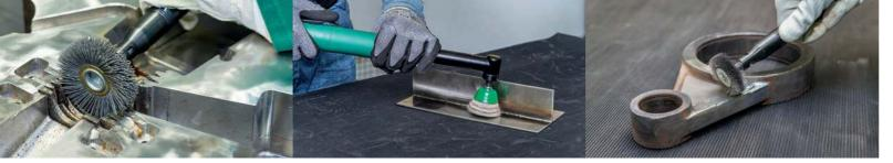
Brushes are highly effective on edges and protruding material - without significantly changing the actual contour of the workpiece. This makes them an excellent deburring and cleaning tool.
