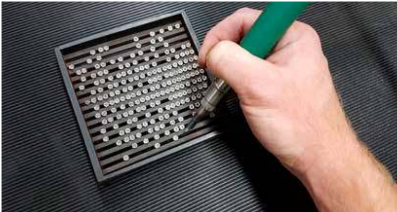
You can pick up screws either using a screw feeder or a simple tool like the rack shown above.
