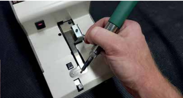
You can pick up screws either using a screw feeder or a simple tool like the rack shown above.
